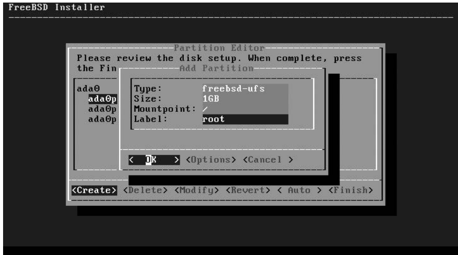
Figure 3-13: Adding the root partition
